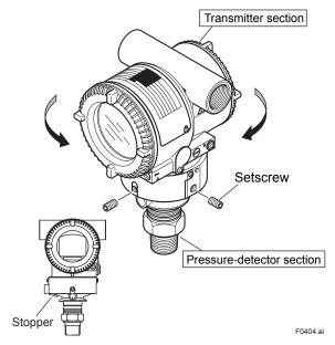
Figure 4.4 Rotating Transmitter Section
