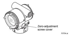
Figure 7.4 External Zero-adjustment Screw
