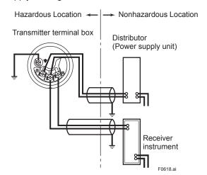
Figure 6.12 Connection between Transmitter,
