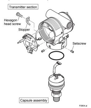
Figure 8.4 Removing and Mounting the Pressuredetector Section
