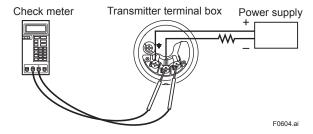
Figure 6.7 Check Meter Connection
