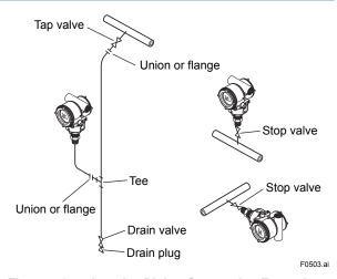
Figure 5.3 Impulse Piping Connection Examples
