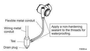
Figure 6.13 Typical Wiring Using Flexible Metal
