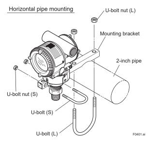
Figure 4.1 Transmitter Mounting
