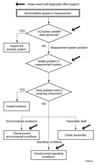
Figure 8.5 Basic Flow and Self-Diagnostics
