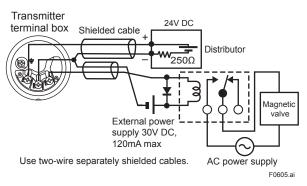
Figure 6.8 Status Output Connection
