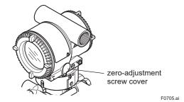
Figure 7.5 Zero-adjustment Screw
