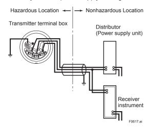
Figure 6.11 Connection between Transmitter, Distributer and Receiver
