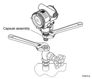
Figure 4.3 Tightening Transmitter
