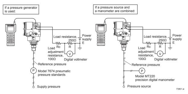
Figure 8.1 Instrument Connections (4 to 20 mA output)
