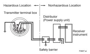
Figure 6.10 Connection between Transmitter and Distributor
