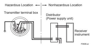
Figure 6.9 Connection between Transmitter and Distributor
