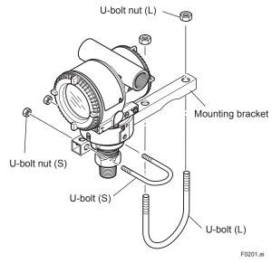
Figure 2.1 Transmitter Mounting Hardware
