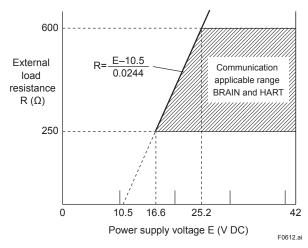
Figure 6.17 Relationship between Power Supply Voltage and External Load Resistance
