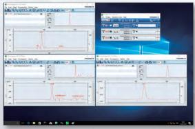
by accurately assessing and displaying the KPIs of each analyzer through real-time data acquisition combined with statistical quality control (SQC) analysis. It also provides a common graphical interface for all the plant's analyzers for validation checks and alarm reporting.
