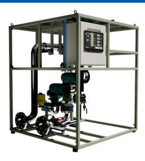
The Rotamass RCx38 are positioned on the main metering lines. There can be 1 to 10 metering lines, depending on the flow range to be measured. These Rotamass therefore measure the general flow and the density of the mixture. By using the density of the three-phase mixture with the densities of the known liquid and gas phase, we then obtain the GVF, or the % of the gas phase in the fluid, at flow conditions P and T.
