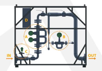
In the by-pass line equipped with the small Coriolis (B) it will measure the liquid density and this is called the water cut line.
