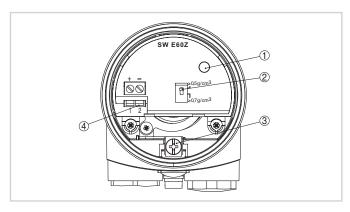
Electronics and connection compartment, single chamber housing
