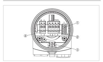
Electronics and connection compartment, single chamber housing
