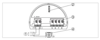
Electronics and terminal compartment, single chamber housing
