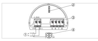
Electronics and terminal compartment, single chamber housing
