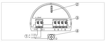
Electronics and terminal compartment, single chamber housing
