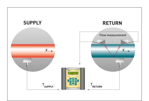
FLUXUS® F601 Energy measures the thermal energy consumed by a system by determining the heat or cold flows entering and exiting it (difference method). For doing so, temperature measurements at the supply and return lines as well as the measurement of the volume flow through the system are required. FLUXUS® uses the measured values to calculate the thermal energy flow based on the heat transfer media's enthalpy curves stored in the internal memory.
